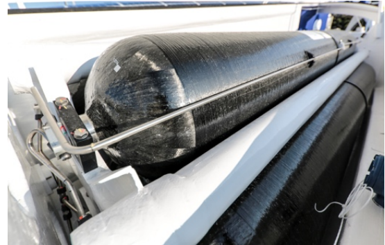
Hydrogen storage tanks
